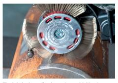
The bristle tips strike the surface, with kinetic energy, resulting in both corrosion removal and micro-indenation in the surface.
